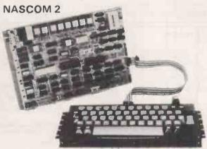
Kit includes all parts to build CPU board which has resident 8K microsoft BASIC and 2K NAS-SYS 1 monitor for machine code programming. Included with kit is a fully assembled LICON QWERTY SOLID STATE KEYBOARD specially designed to exploit the potential of the NAS-SYS monitor. Other interfaces include video to monitor or domestic TV. Kansas City standard cassette interface (300/1200 baud) or RS232/20mA teletype interface. In addition to full character generator graphics ROM is provided to give
